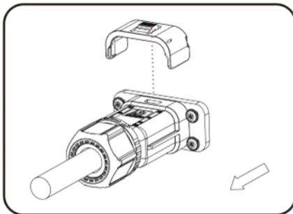
Use a tool to point at the unlocking position, hold the cable driver, and pull it back to separate the male and female
