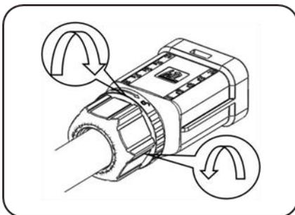
Hold the unlocking buckle with one hand and rotate it in the direction indicated, while rotate the nut in the opposite direction with the other hand
