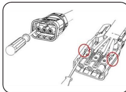
Remove the red circles on both sides using a screwdriver
