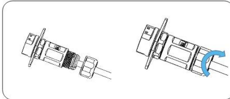
Note: Make sure the Meter communication cable is to the right position on the inverter (refer to 5.5)
