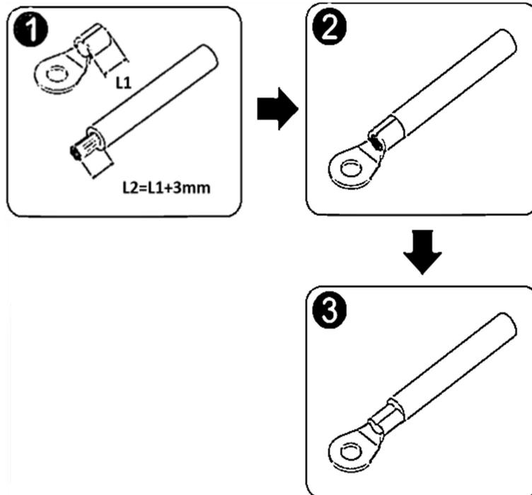
Procedure 2 connect the premade ground cable to the right position (shown on the following picture) and make it is fixed tightly.
