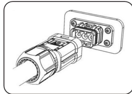
The female connector is separated from the board connector
