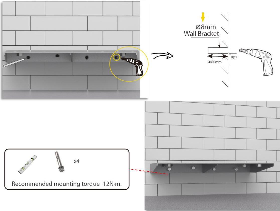
Install the base on the Wall-mounting pallet, and then install the positioning plate.
