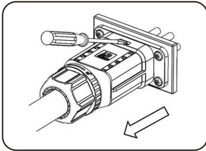
Use a screwdriver to point at the unlocking position, hold the cable driver, and pull it back to separate the male and female
