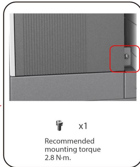
Repeat step3 until you have installed all the battery modules of battery packs.
